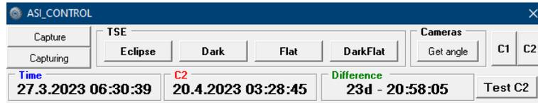
Buttons Capture and Capturing are use for test images making. This images are taken with both cameras simultaneously.
